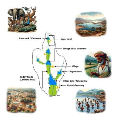
Each tank in a given cascade system adopts geographical and functional features to harmonise with nature. The functional components of a tank perform specific purpose and roles of these components are explained below.
